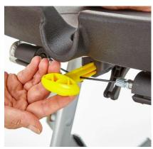
Pull the Yellow handle on the rear of the seat to unlock the seat.
