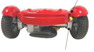
Up = Freewheel Mode (Motor is Disengaged)
