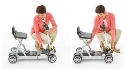
Lift up the floorpan in the centre at the point indicated in Yellow and slide the front wheels towards the rear.
