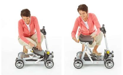
Tip the rear of the seat slightly upwards and lift the whole seat up to lock in the open position.
