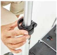
When the tiller is in the desired position close the Tiller Adjustment Clip until it is as tight as possible.
