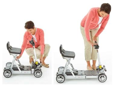
Pull the front wheels forwards until the floorpan is flat.
