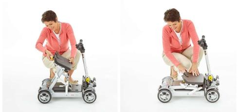
Tip the front of the seat slightly forwards and push the whole seat downwards to lock in the closed position on the floorpan.
