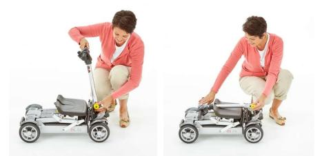
Pull the Yellow Tiller Adjustment Knob and push the tiller down to lock into the seat in the closed position.
