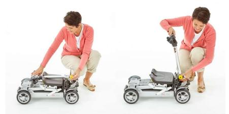
Pull the Yellow Tiller Adjustment Knob and lift the tiller up to lock into the upward position.
