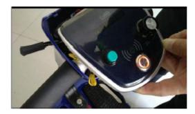
Place key fob on power button then briefly press the green 'Horn' button once. Keep the key fob on the power button until you hear a beep and light will turn blue.
