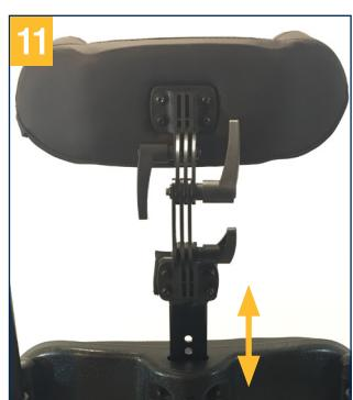
Let go of the locking knob and pull the headrest up until it snaps into the first position. Now, by pulling the locking pin outwards again and simultaneously pulling upwards, you can change the height of the headrest. Make sure that the locking knob snaps into the selected position. (Fig. 11).
