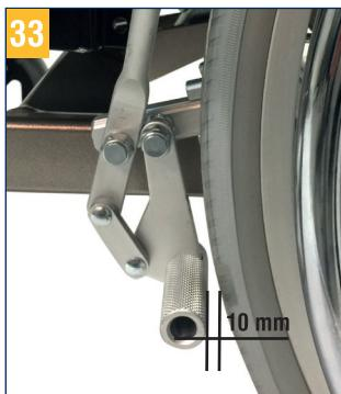
The interval between the center mounting bolt and the tire cover must be 10 mm at the narrowest place when the brake mechanism is opened at its maximum.
