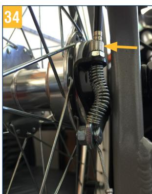
To achieve an optimal braking effect, the braking force is adjusted with the adjusting screw.
