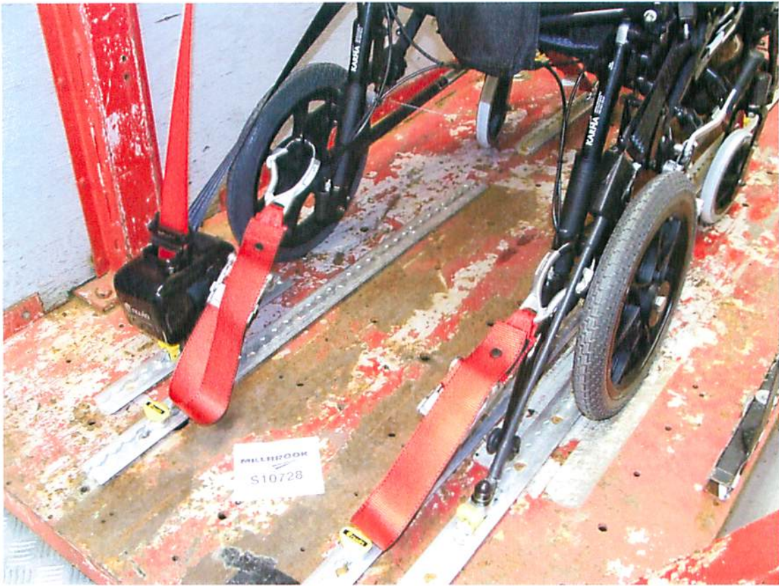
Rear wheelchair restraints, pre-test
