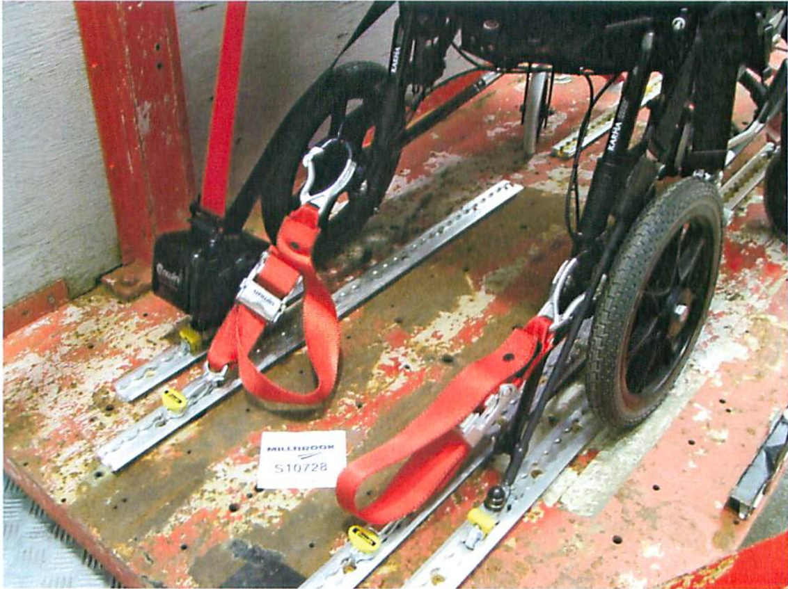
Rear wheelchair restraints, post-test
