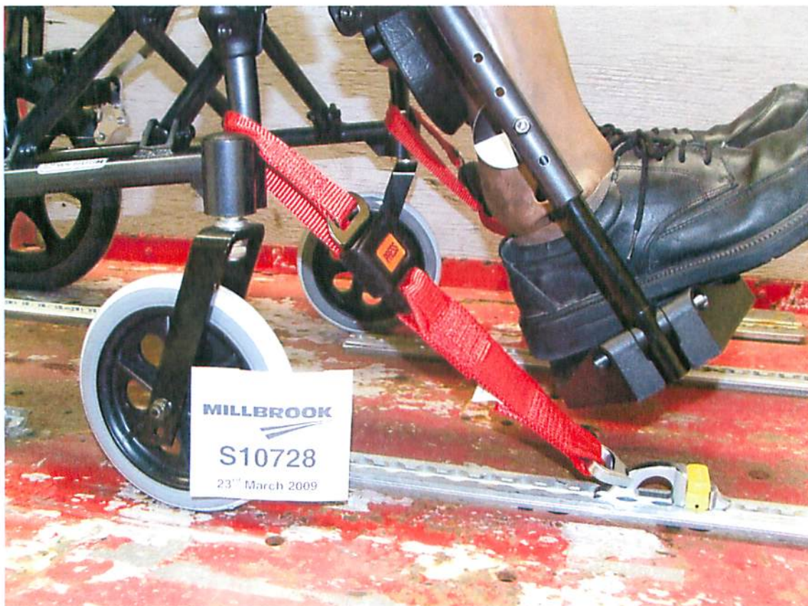
Front wheelchair restraints, pre-test
