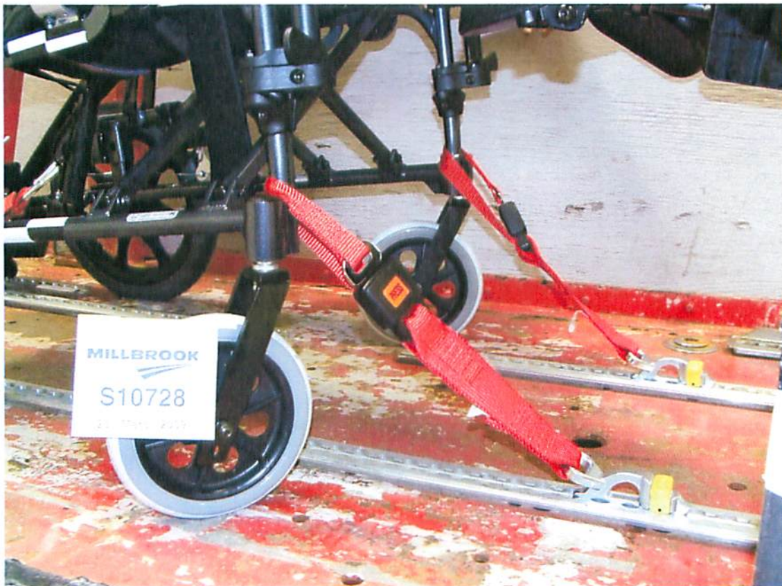
Front wheelchair restraints, post-test
