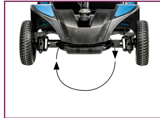
37" turning radius (15% smaller than that of the Elite Traveller)
