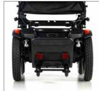
Larger 14" drive wheels and 9" front castors for better kerb-climbing and handling of outdoor terrain.
