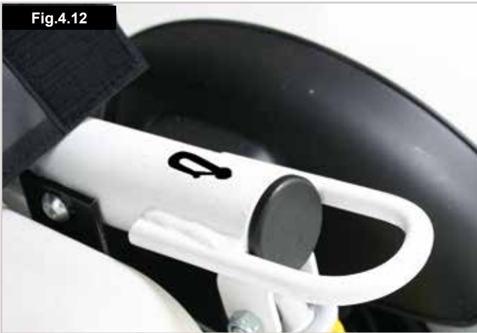
Position of the Rear tie down label & bracket, (Fig.4.12).
