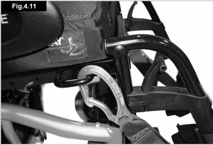
Position of the Front tie down restraint., (Fig.4.11).
