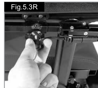
SALSA R2 & M Below-from August 2010 (Fig.5.5 - 5.8) By rotating the red lever outwards on both sides of the motor the brakes are released from the motors.
