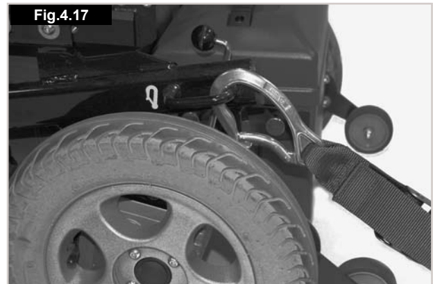
Position of the Rear tie down restraint on latest Rumba and Rumba Modular, (Fig.4.17).
