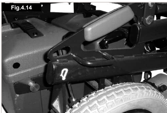
Position of the Rear tie down label & bracket on original Rumba (Fig.4.14).
