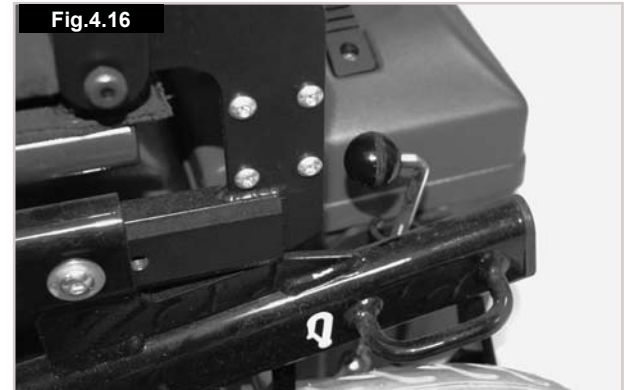
Position of the Rear tie down label & Bracket on latest Rumba and Rumba Modular, (Fig.4.16).
