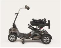
Once the tiller is clear of the seat place the other hand under the seat and continue to pull both until the Maximo is fully open as shown below. Then lift the back of the seat and rotate the arm rests forwards.
