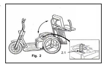
**Batteries** – For safety in transit the main supply leads may have been disconnected from the batteries. The black lead would have been disconnected from one battery and the red lead from the other. These will be taped to the batteries in an obvious position as will the fixing bolts. Simply reconnect the leads ensuring the bolts are correctly tightened.
