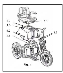
Removal and Replacement of Deluxe seat – To remove seat, release the seat locking lever, at front of seat, and turn seat through 180° so that it faces to the rear. Now lift seat straight up and out. Replacing the seat is just a reversal of the above.
