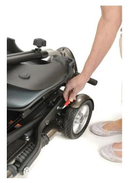
2. Pull the tiller away from the floor pan until the front wheels of your Minimo Plus touch the floor.
