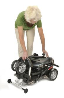
Once folded you can then lift your Minimo Plus using the handle at the rear and stand it on its front wheels to move around in the folded position.
