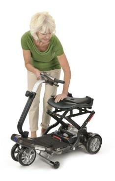
4. Finally push the tiller against the seat and the front of the floor pan towards the rear wheels to ensure your Minimo Plus is locked into the folded position.
