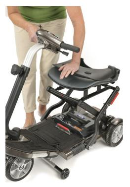
3. Use one hand to push the seat down towards the floor pan and the other to move the tiller towards the seat which will lift the front wheels off the floor and fold your Minimo Plus.
