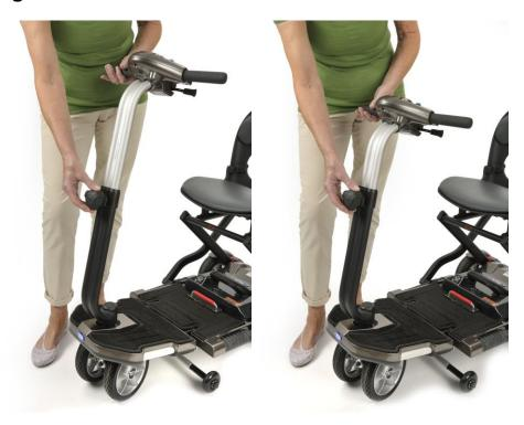
If you'd like to adjust the height of your Minimo tiller simply turn the adjustment wheel anti clockwise until the top part of the tiller moves freely up and down. Then just move the top half of the tiller to the height you would like and tighten the adjustment wheel by turning it clockwise until tight.
