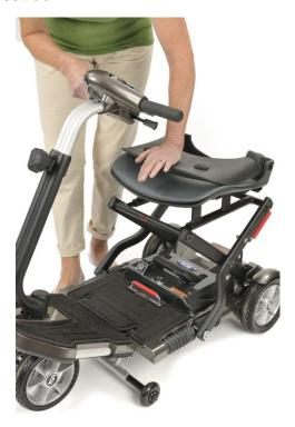
3. Use one hand to push the seat down towards the floor pan and the other to move the tiller towards the seat which will lift the front wheels off the floor and fold your Minimo.
