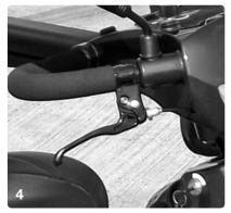
system is controlled by pulling/compressing the lever on the right hand side of the handle bars/ tiller (Fig.4). The more pressure you apply to the lever the heavier the braking effect will be.
