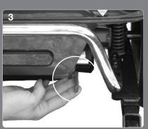
The Freewheel device allows the vehicle to be pushed without power. To activate, first locate the lever (Fig.3). When standing behind the scooter, it is located on the right hand side of the rear of the vehicle - See Illustration.
