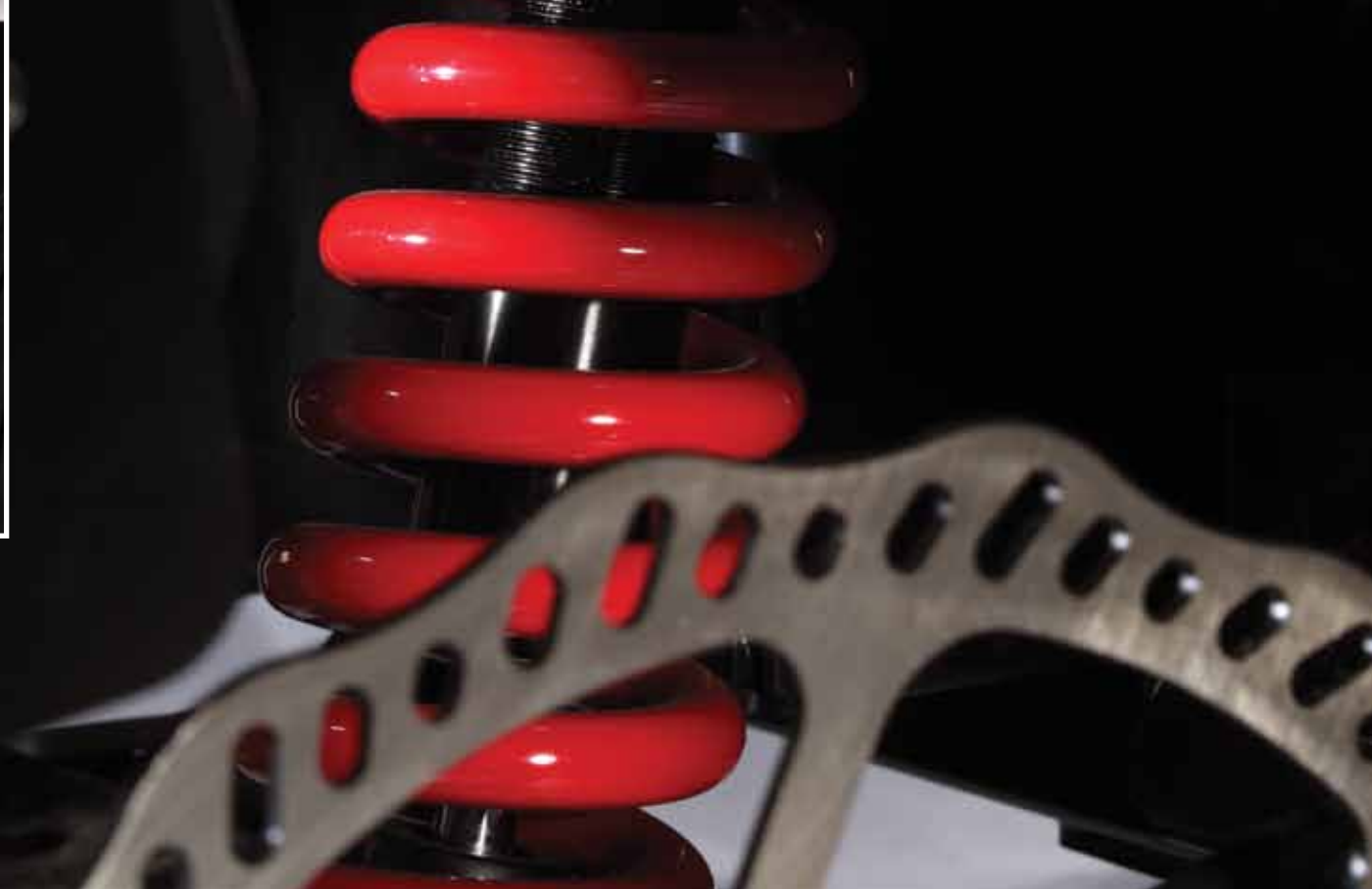
Rear mono shock single suspension for even greater comfort
