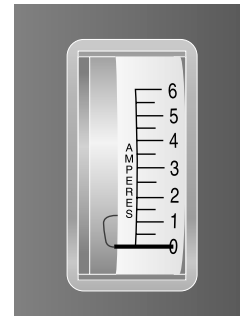
FIGURE 8. AMMETER INDICATES BATTERY IS FULLY CHARGED
