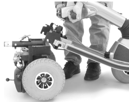
FIGURE 20. SEPARATING THE FRAME SECTIONS
