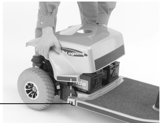
FIGURE 14. REMOVING THE REAR SHROUD
