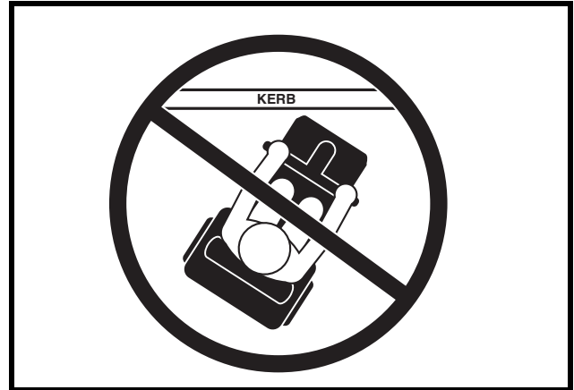
Figure 3A. Incorrect Kerb Approach
