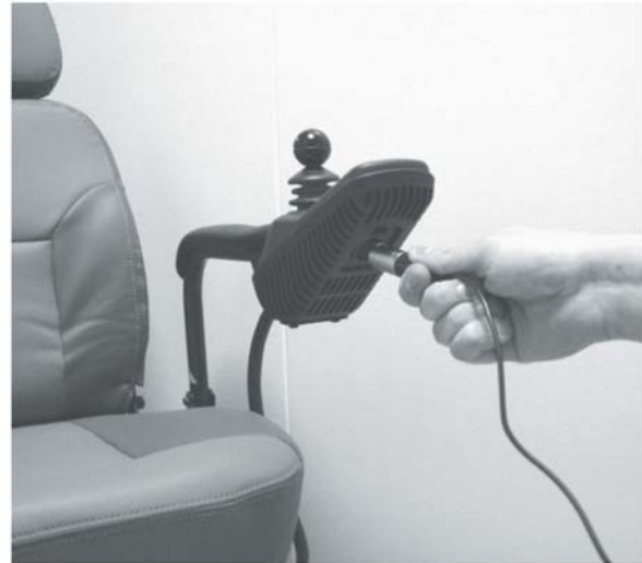
Figure 6 — Joystick Controller Charger Connection
