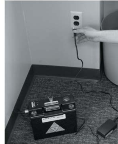
Figure 5a — Battery Pack Charging Connection (Removed from Power Chair)
