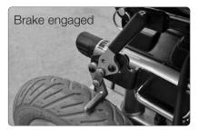
engage. This will stop the vehicle rolling forwards or backwards. When you start, this brake will automatically disengage. If the battery should go flat this brake automatically engages. The P200 is also fitted with a handbrake on each of the the rear wheels. Push the lever forward to engage each brake. Never leave the powerchair in freewheel without engaging **both** brakes. Both brakes should be engaged before you get on or off the powerchair.
