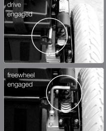
• Move both the levers to engage drive. The vehicle is now braked. This is the normal operating position.
