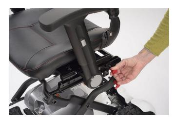
2. Slide the seat forwards slightly and lift away from the base.
