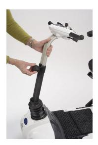
If you'd like to adjust the height of your tiller simply turn the adjustment wheel anti clockwise until the top part of the tiller moves freely up and down. Then just move the top half of the tiller to the height you would like and tighten the adjustment wheel by turning it clockwise until tight.
