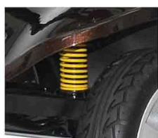
Suspension for more comfortable driving
