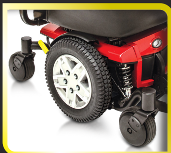
Mid-Wheel Drive design, which is ideal for tight turning circles
