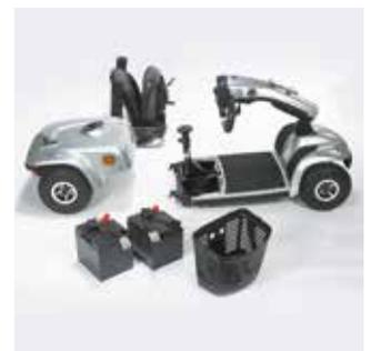
**Disassembly into five parts**
