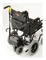
This wheelchair is suitable for some retrofit powerpacks, such as the PowerStroll. A suggested configuration is shown left.
