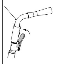
Push the black paddle (arrowed) towards the back post with your thumb whilst pulling the handle down. Repeat this operation for the other handle. To put the backrest back into position, lift both handles together and the folding mechanism will lock back automatically.
