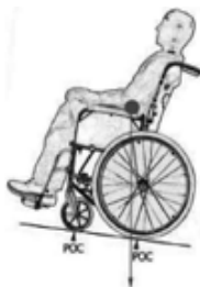
Figure 5 Stable on slope
