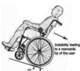
Figure 6 Unstable (slope too steep)
