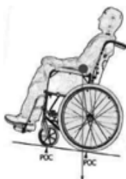
Figure 5 Stable on slope
