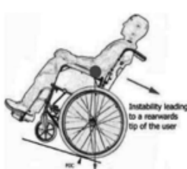
Figure 6 Unstable (slope too steep)
